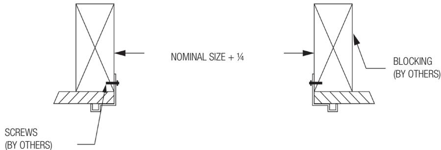
**Step 3:** Refer to Page 7 for concealed mounting component breakdown and how to install concealed mounting bracket onto the grille and into the mounting frame.
