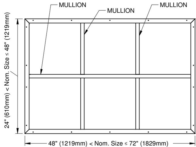
ALL METRIC DIMENSIONS ( ) ARE SOFT CONVERTED. IMPERIAL DIMENSIONS ARE CONVERTED TO METRIC AND ROUNDED TO THE NEAREST MILLIMETER.
