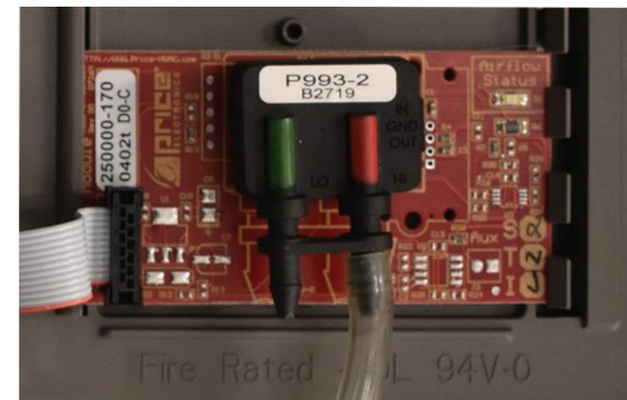
Static Pressure Probe connected to **HI Side** of transducer. LO side left open to atmosphere.
